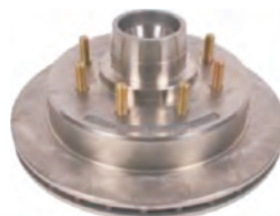
ROTOR/HUB-133-7-8 13" Rotor Integral w/Hub (Standard Automotive Finish) Fits 865 wheel bolt pattern with 1/2" wheel bolts #25520 and #14276 bearing cup (34 lbs)
