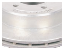
Dacromet coating offers the best value of protection for salt water applications (i.e. during a standard salt spray test, rust will begin forming between 300 and 400 hours).
