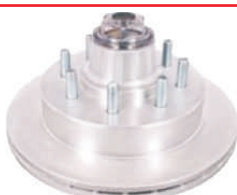
ROTOR/HUB-133-8-9-DAC 13" Rotor Integral w/Hub (Dacromet Coated) Fits 865 wheel bolt pattern with 9/16" wheel bolts #25520 and #02420 bearing cup Must use 8k outer bearing (40 lbs) *8K rotor
