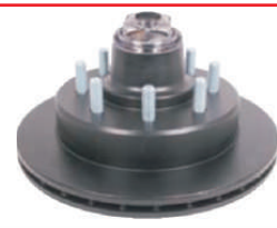
ROTOR/HUB-133-8-9-E 13" Rotor Integral w/Hub (E-Coated) Fits 865 wheel bolt pattern with 9/16" wheel bolts #25520 and #02420 bearing cup Must use 8k outer bearing (40 lbs) *8K rotor
